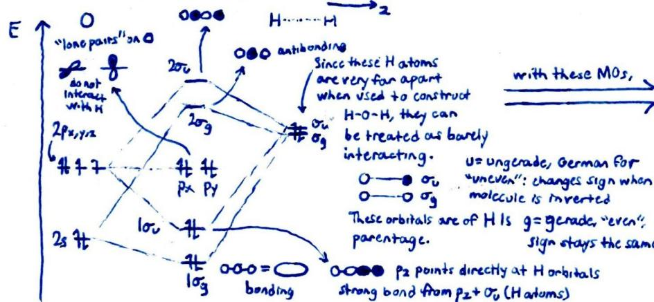
For real calculations, the intrinsic energies of atomic orbitals (which key us in on the relative energies of H and orbitals) come from "valence orbital ionization energy" tables describing how tightly bound various  $e^-$  are. These can be found in textbooks and online.
